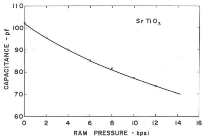
Fig. 15 Capacitance versus ram pressure for single crystal SrTiO<sub>3</sub> measured at room temperature
